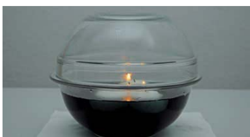
Figure 3 and 4: The bowl with the burning candles is covered with a second bowl. After several minutes, the candles burn out.
