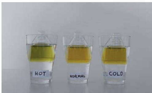
Figure 4: The green shade indicates that the water in the bottle with the hot water bath has already released \text{CO}_2 back into the air.
