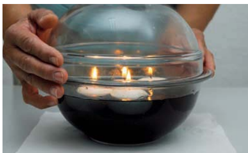
Figure 2: Four burning candles float in the bowl with green indicator.
