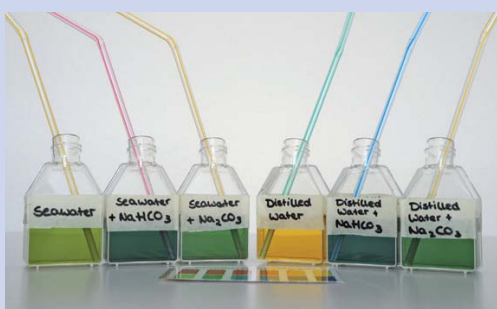
Figure 2: The colour of the water after blowing into the bottles for 20 seconds.
