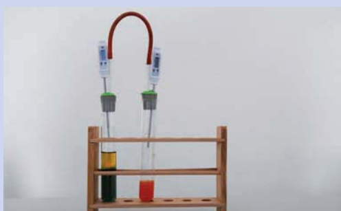
Figure 5: Change of colour after the addition of the first quarter of an effervescent tablet.
