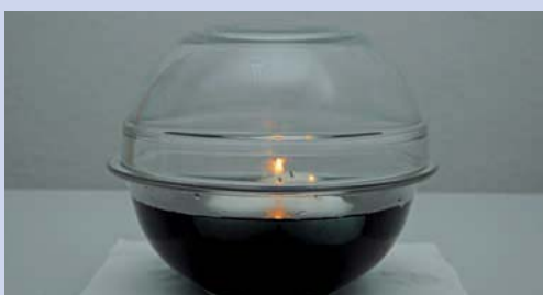
Figure 2: Four burning candles float in the bowl with green indicator.
