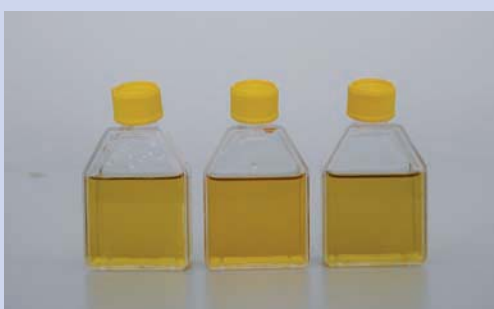
Figure 2: CO 2 was added by blowing air into the bottles. The yellow colour indicates that the water became more acidic.
