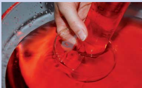
Figure 1: Covering the cylinder mouth with a petri dish.
