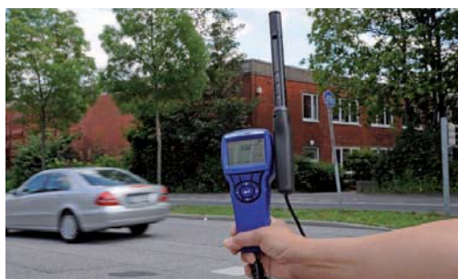
Figure 1: In order to practice the handling of the CO 2 analyser you can measure the air at various locations around the school and inside the building.
