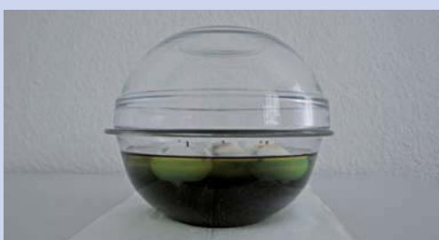
Figure 3 and 4: The bowl with the burning candles is covered with a second bowl. After several minutes, the candles burn out themselves.
