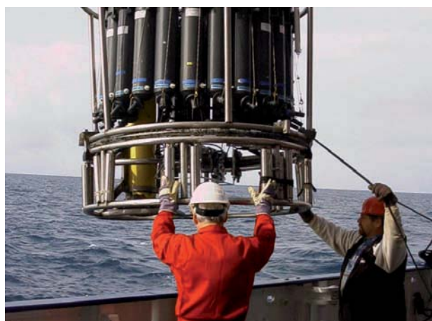
Figure 3: Marine scientists also record the pH of the oceans using probes attached to a rosette water sampler.
