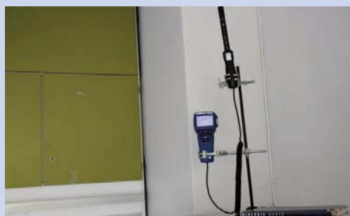
Figure 1: The CO 2 sensor is mounted on a stand and held with a clamp on a cupboard at the back of the classroom. This way the pupils are not distracted. Ensure free air circulation around the sensor.
