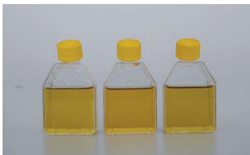
Figure 2: CO 2 was added by blowing air into the bottles. The yellow colour indicates that the water became more acidic.
