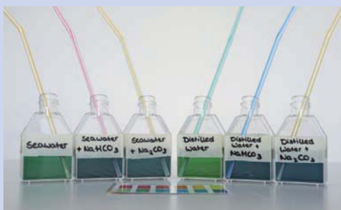
Figure 1: The six bottles after the indicator is added.
